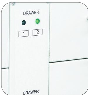
3. Once the box arrives, a green light indicates the drawer is unlocked and can be opened. Only one drawer can be accessed at a time.
